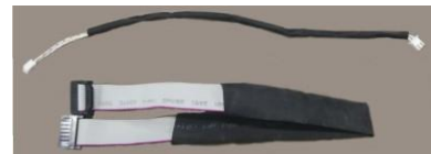
cables between Parallel card and control board,main board
